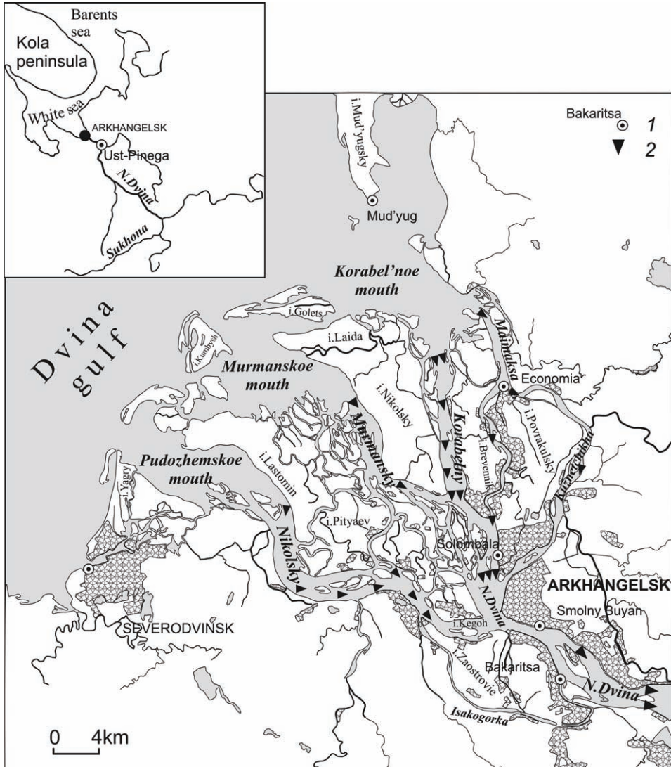
Figure 1. The cartographic scheme of the delta of the Northern Dvina River. 1 – gauging stations, 2 – reaches of periodic forming the ice dams
